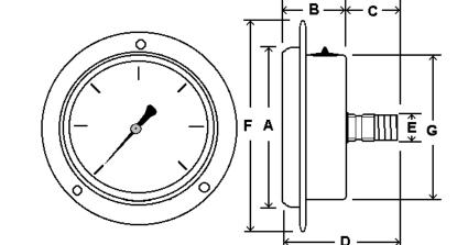
Design meets or exceeds ASME B40.100 pressure gauge standard.
